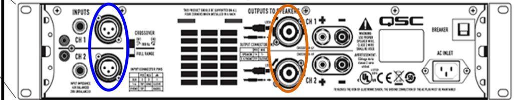
Use short XLR (microphone) cables to connect Snake 13 to Amp Input 1 (feed for MAIN speakers) and Snake 14 to Amp Input 2.
