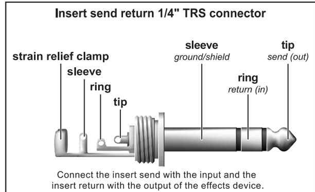
Fig. 4.4: 1/4" TRS connector for insert send/return applications
